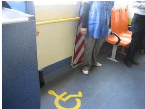
photo 2-5-10 space for wheelchair users on the ultra low-floor bus
