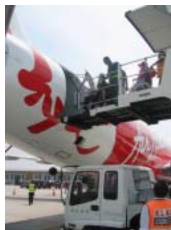
Photo 2-5-12 Lifting a passenger onto an aircraft (2)
